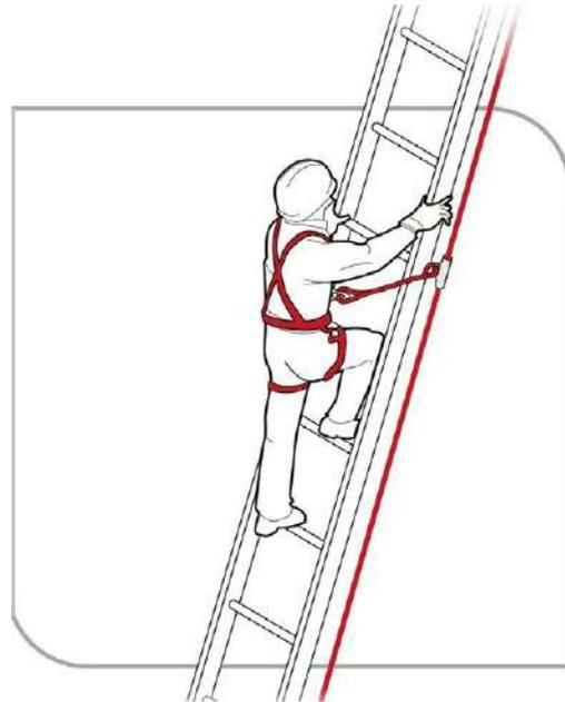
Figure 6: Anchorage line system for ladder use
