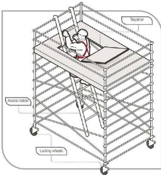
Figure 2: Mobile scaffold with access ladder and trapdoor
