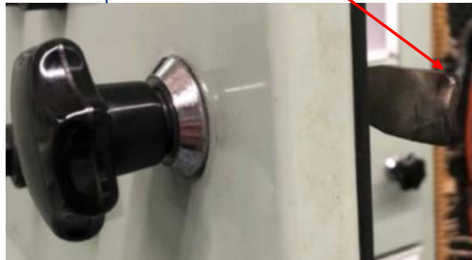
Two views of the door latch tongue. - From behind showing the arc burn - From the front showing the burn mark on the lip
