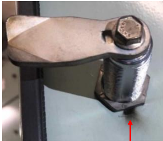
Two views of the door latch tongue. - From behind showing the arc burn - From the front showing the burn mark on the lip
