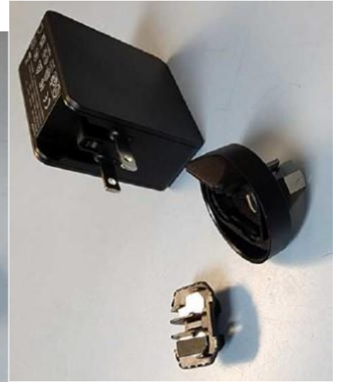
2 views of how the adapter was found with the top cover separated from the base leaving the pins exposed
