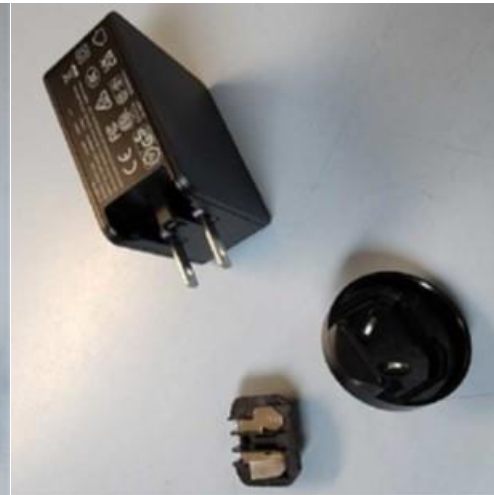
2 views of how the adapter was found with the top cover separated from the base leaving the pins exposed
