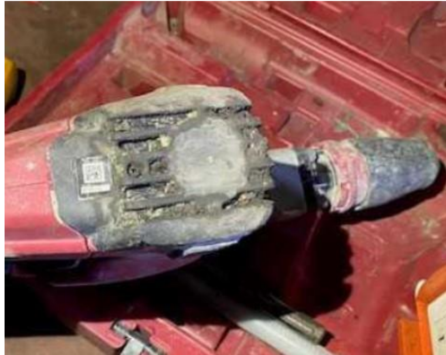
A close up of the base of the drill. Note all the moist dirt build up inside the slots. Some of the slots are vent hole which have allowed moisture to enter the drill
