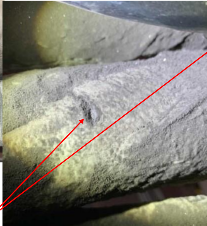
Minor damage to the cable sheath evident after removal of the ablative coating.
